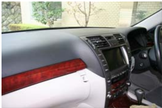
For the instrument panels of automobiles (Thermoplastic polyurethane beads for the interior parts of automobiles)
